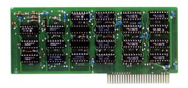
16K memory expansion card for the Apple II and II+ fully compatible with Applesoft, CP/M and Pascal. Plugs into slot 0.
