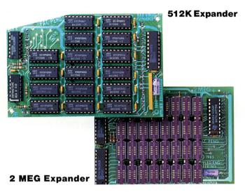
Should you ever run low on memory with Ram-Works II (unlikely) you can add these expander cards to your RamWorks II at any time. And of course, the above expander cards are compatible with the original RamWorks too.
