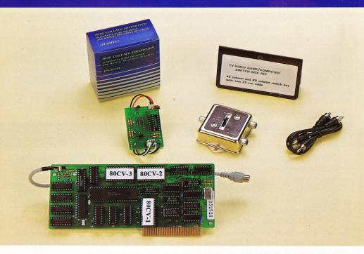
The 80 Column Expander provides sharp 80 column text by 24 lines for your Apple II, II+, or Franklin Ace, computer.
