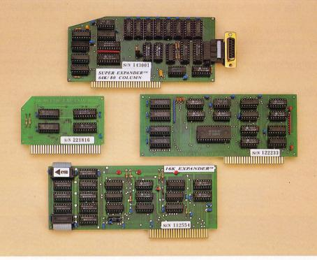
Since many Apple users do not require a large memory bank for operational use, a smaller set of EXPANDER RAM boards has been created. The Expander RAM boards have the same quality & advanced design as the Super Expander RAM boards, only less memory & more affordable pricing.
