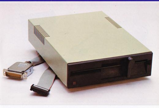
This 5¼ slimline disk drive is fully compatible with all Apple software including DOS 3.2, DOS 3.3, ProDOS, CP/M, and PASCAL. The drive can be used as a direct replacement for your primary drive, or as an add on secondary drive.
