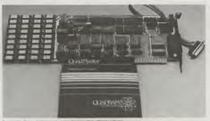
Quadboard II offers six function on one card and comes with QuadMaster software.
