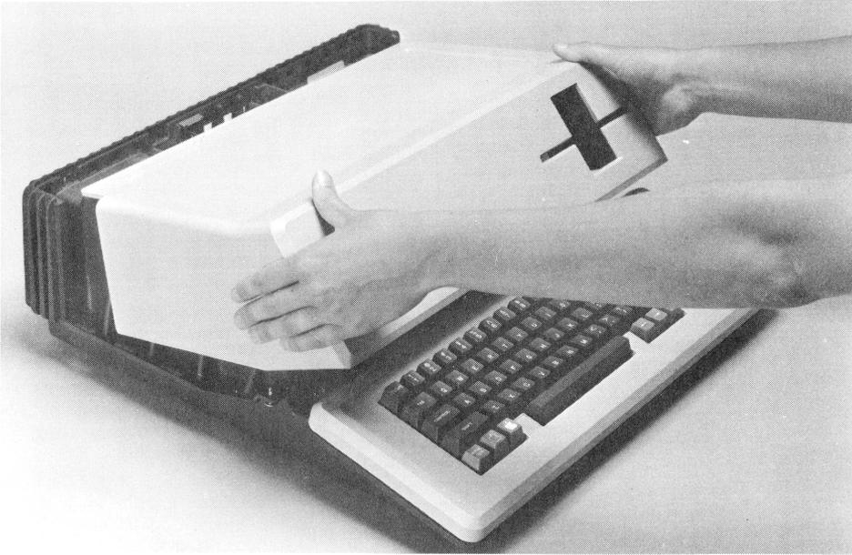
Figure 2-5. Removing the cover
