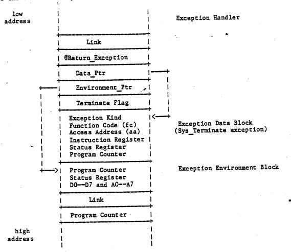
The Exception Data Block given here reflects the state of the stack upon a SYS\_TERMINATE exception. The term\_ex\_data record described in the Interface appendix gives the various forms the data block can take. The status register and program counter values in the data block reflect the true (current) state of these values. The same data in the Environment block reflects the state of these values at the time the exception was signalled, not the values at the time the exception actually occurs.
