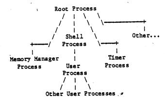
Any other system process (the Network Control Process, for example) is a son of the root process.
