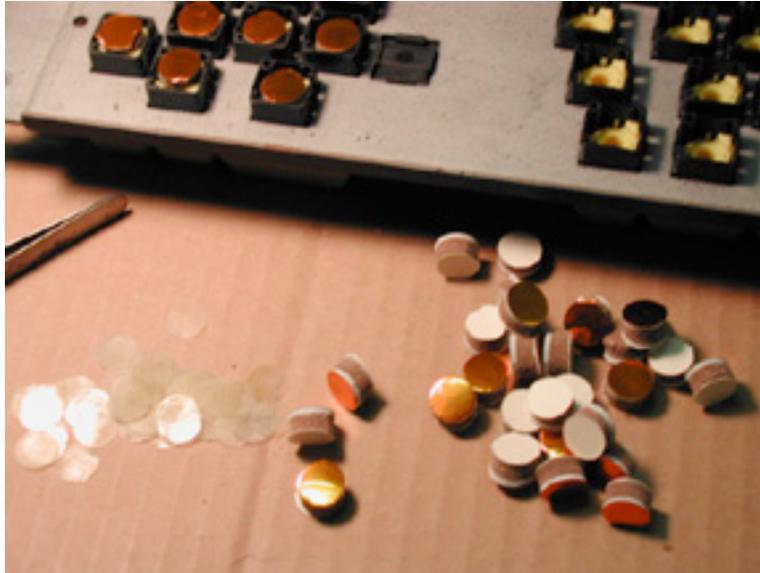
Replacement of the foam pads in progress on my first attempt to replace the pads. Note that the pads shown proved to be too thick and not resilient enough for a good keyboard feel. The procedure given in this document will produce pads with a good feel.
