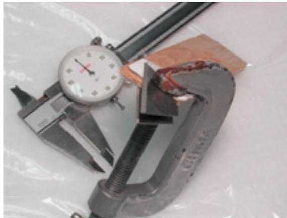
Two box-cutter blades were held with a c-clamp so that they sandwiched an ~.2" shim. The resulting foam was of inconsistent thickness. I recommend avoiding this procedure by purchasing 3/16" foam.
