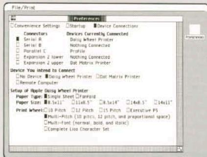
*Printer set-up options—such as paper size and type, and print wheels—are all controlled from within Lisa applications. Simply point with the mouse to select each option.*
