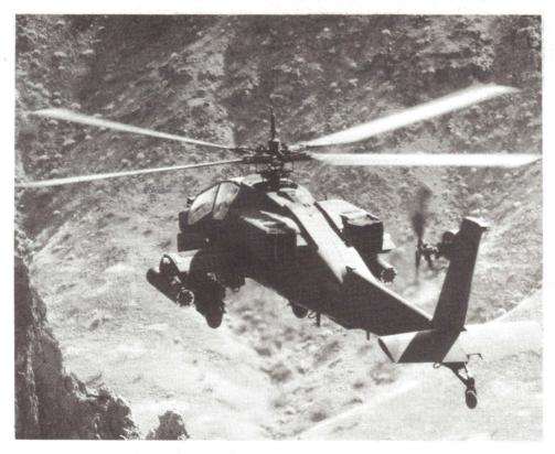
Capable of hovering on both engines at 65% torgue and 106% from a single engine, the Apache crew can be confident to survive a single engine failure, even in the hover.
