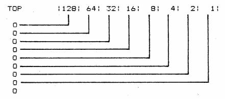
NOTE: DUE TO THE FACT THAT A CHARACTER IS MADE UP OF 8 DATA BITS. THE BOTTOM NEEDLE OF THE PRINT HEAD CAN NOT BE ADDRESSED.
