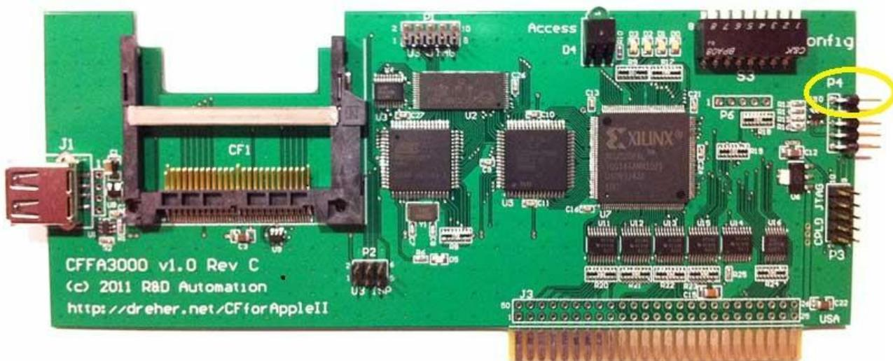
Figure 13: CFFA3000 connector to remote P4 pin 1 location
