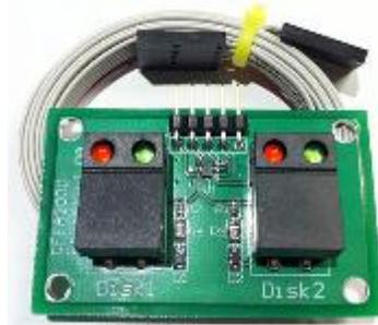
Figure 15: Remote pushbutton board.
