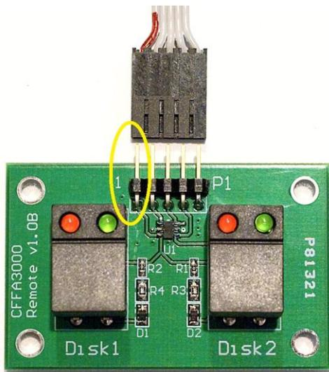
Figure 12: CFFA3000 Remote connector P1 pin 1 location
