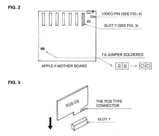
Locate the video output connector on the rear of the computer cabinet. Directly in front of this connector is a short row of electrical components, and then a row of four vertical pins which are located nearest to the video jack. Connect the video cord from the RGB-IIB module to the second pin from the right end of this row, as shown in Fig. 4. Connect the end of video cord with the four pin plug of RGB-IIB to the video pin of the APPLE-IIPLUS computer.
