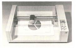
only have to issue a MA (move absolute command) to the plotter to move the pen to a location you desire. For the example the upper left corner of box #1 is at 200,1500 so you would enter MA200,1500 {Moves to 200,1500} DR500,0,0,-200,-500,0,0,200 {Draws our box}
