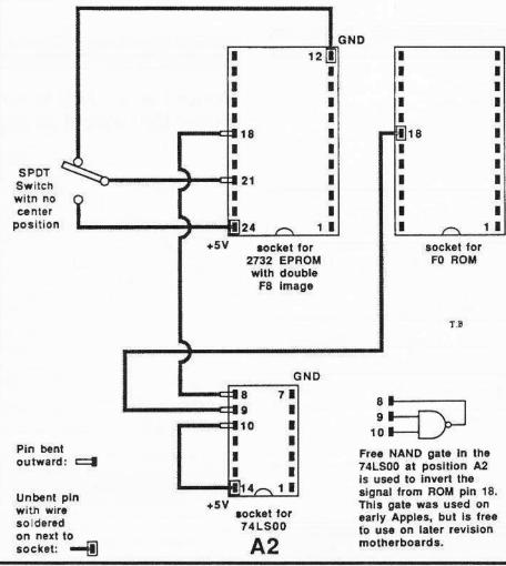
The 2732 EPROM requires a signal to pin 18 (ROM inhibit) which is inverted as compared to the signal required by the ROMs used in the Apple II.
