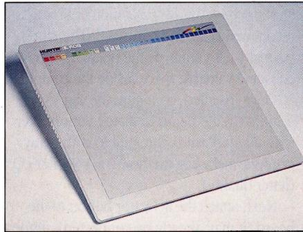
*This digitizing pad from Kurta enables the creator to draw more precisely than is possible with a mouse.*
