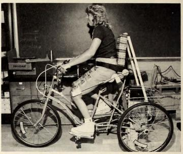
Nan Davis provides the motive power for the outdoor tricycle. The more complicated movements required to ride the "Zap Bike," as it is affectionately called, are controlled by a Z-80 microprocessor running an assembly language program developed by Petrofsky on the Apple.
