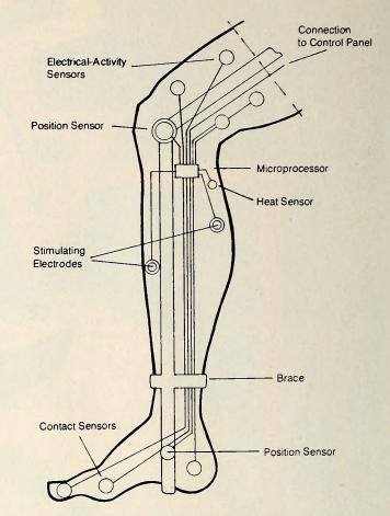
Blueprint for mobility: The microprocessor just below the knee accepts feedback input from contact, heat, electrical activity, and position sensors placed at strategic locations on the leg brace and the leg itself. The microprocessor stimulates muscles of the lower leg through electrodes.
