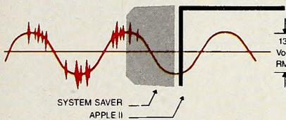
By connecting the Apple II power input through the SYSTEM SAVER, power is controlled in two ways: 1) Dangerous voltage spikes are clipped off at a safe 130 Volts RMS/175 Volts dc level. 2) High frequency noise is smoothed out before reaching the Apple II. A PI type filter attenuates common mode noise signals by a minimum of 30 dB from 600 khz to 20 mhz, with a maximum attenuation of 50 dB.
