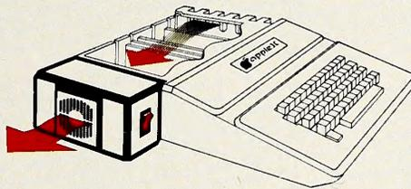
SYSTEM SAVER provides correct cooling. An efficient, quiet fan draws fresh air across the mother board, over the power supply and out the side ventilation slots.
