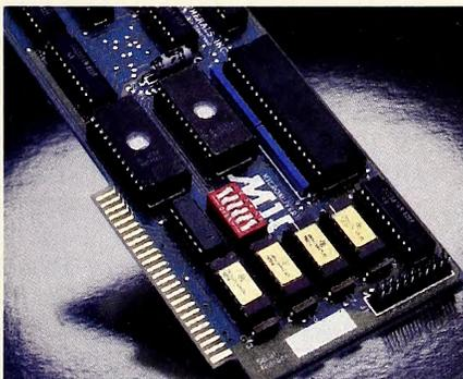
computer. An intelligent interface card with up to 32K of RAM for data buffering, Microbuffer II features on-board firmware for text formatting and advanced graphics dump routines. Both serial and parallel models have energy-efficient low power consumption coupled with a high data transfer rate. Print formatting functions include Basic listing formatter, self-test, buffer zap, text screen dump, fully programmable control characters and transparent and maintain modes —
