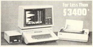
Interactive Microware's general-purpose ADALAB<sup>®</sup> data acquisition and control system interfaces with virtually any lab instrument using a recorder or meter, including GC and HPLC systems, spectrophotometers, pH meters, process control apparatus, thermocouples, etc.
