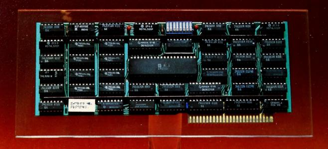
The Accelerator II: Based on a fast 6502 processor with 64K of high-speed memory. Includes built-in fast Language card. Hardware compatible with all standard peripherals. Transparent operation with Apple II software. Special pre-boot diskette included to run Applesoft, PASCAL, and Integer Basic from high-speed RAM. Suggested retail price: \$599.
