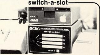
The switch-a-slot connects to any peripheral slot of the computer through an 18" cable. The user can plug up to four cards in the switch-a-slot. The desired card is chosen by using a switch on the front, and only the selected card draws power. This product is suitable for most peripheral cards. The switch-a-slot is perfect for selecting between different printer cards.
