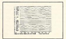
The system is available for Apple II and IBM PC computers. A non-graphics version is available for CP/M 2.2 It uses the network editor to create netlists and text printer plots to display simulation results. All versions require 2- 5 1/4" disk drives.
