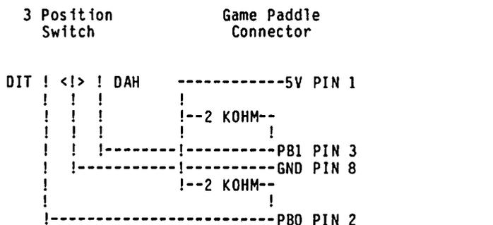
FIGURE 1. Electrical connection of the three position switch is easily achieved via the Apple's game I/O socket. A 16 pin DIP connector should be hooked up as shown.
