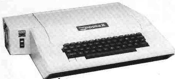
It is well known within the industry that a large proportion of Apple system malfunctions are caused by overheating and power supply switches. The Pact Fan Module eliminates the risk of these problems occurring immediately on installation.
