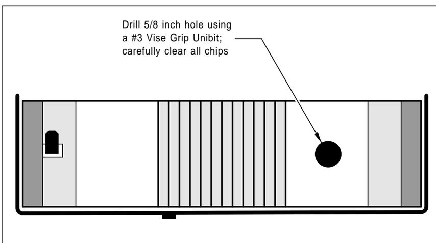
Fig. 3 – Adding a fresh toner filling hole to a *SX* cartridge.
