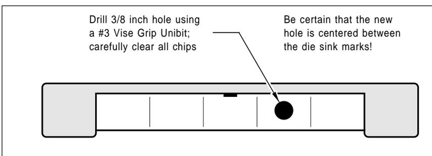
Fig. 4 – Adding the spent toner emptying hole to a *Canon SX* cartridge.
