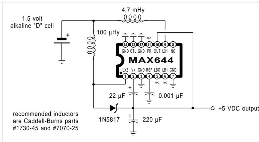
Fig. 2 – This simple switching regulator steps up a single alkaline cell to give you a fixed +5 volt output at 50 Milliamperes. An external pass transistor can be added for more output current.
