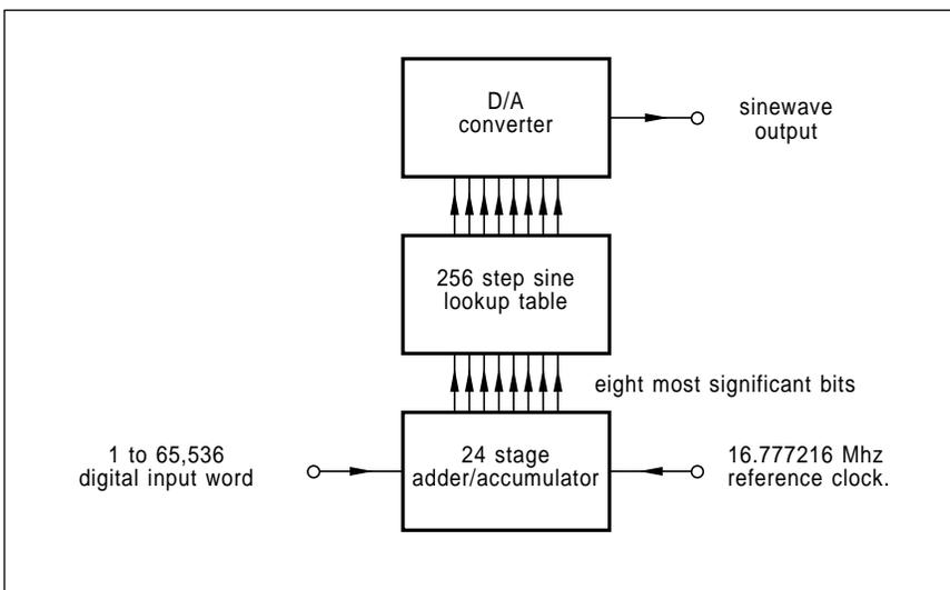
Fig. 1 – Digital sinewaves generated by phase addition. The input word sets how fast the waveform phase will advance, which in turn decides the directly synthesized output frequency. The values shown will generate from 1 Hertz to 65.536 KiloHertz in 1 Hertz steps.
