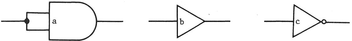
Buffer as (a) Two-input Gate, (b) Buffer and (c) Inverting Buffer
