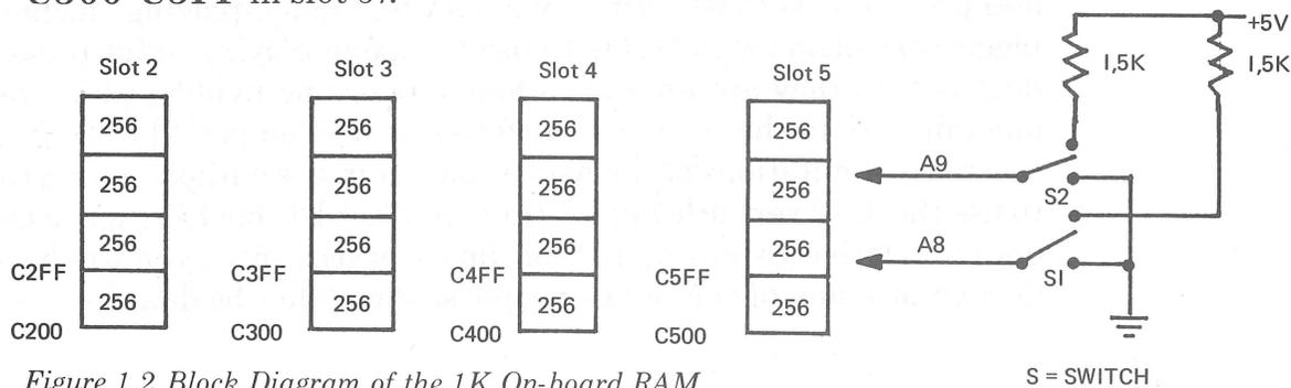
Figure 1.2 Block Diagram of the 1K On-board RAM
