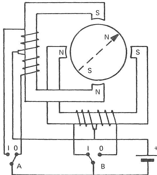
Figure 9.4 Step Motor Movement
