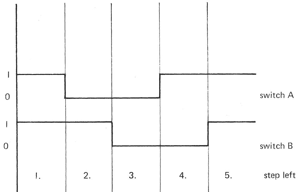
Figure 9.6 Left Turn Timing Diagram
