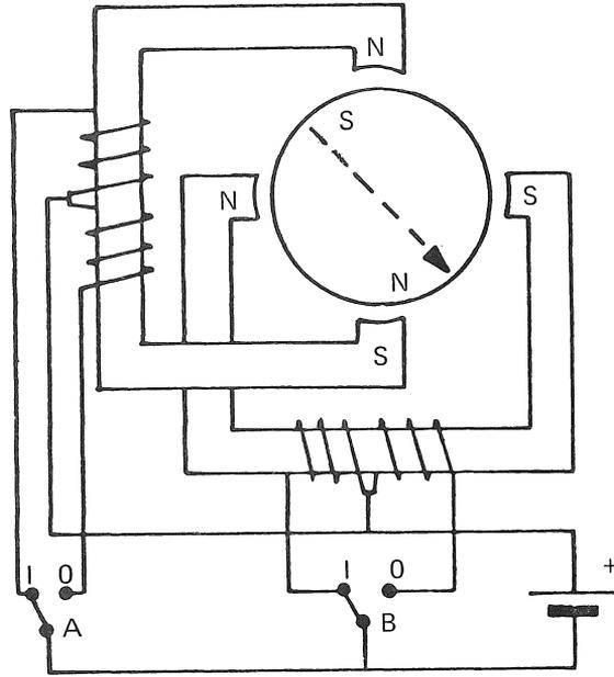
Figure 9.1 Step Motor Movement
