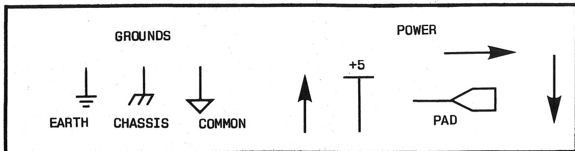
The first are known as grounds, and they are used to indicate a potential of zero or neutral voltage. The first of the trio is an earth ground, commonly used in radio, television and hi-fi schematics, but purist use it only describe an actual connection to a ground spike or cold water pipe. The second is a chassis ground, indicating an electrical connection to the metal case which encloses the circuit. It is often (though incorrectly) interchanged with the earth ground.
