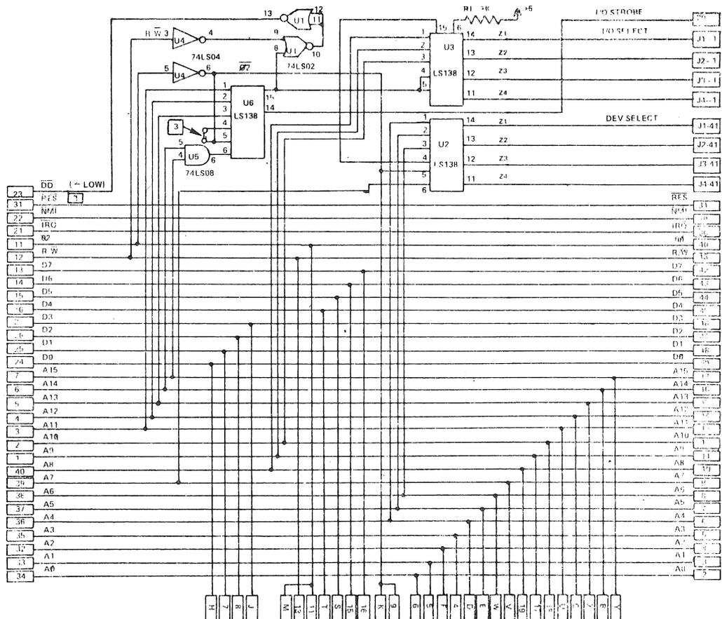
Figure 6.4 The Complete Schematic for the Slot Repeater
