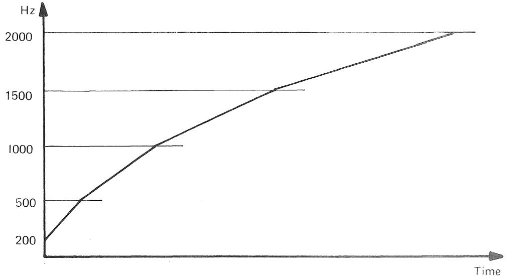
Figure 9.17 Step Motor Acceleration
