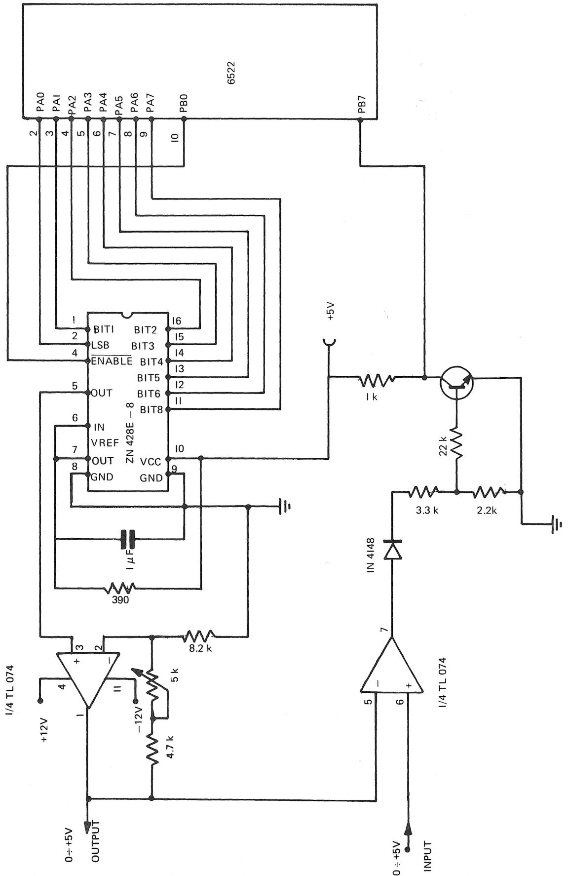
Figure 3.1 8-bit D/A and A/D Converter Schematic
