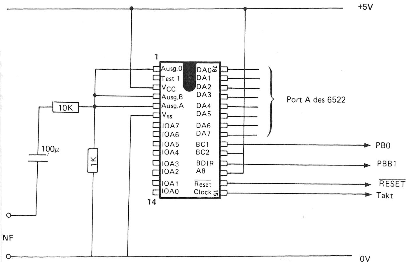
Figure 2.16 Schematic of the Sound Board
