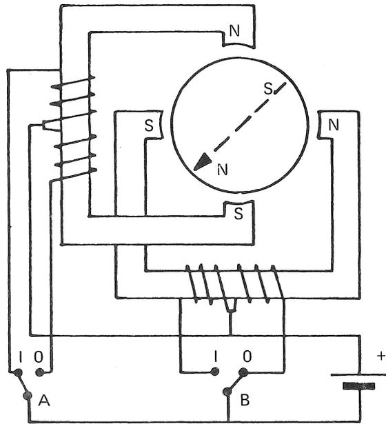
Figure 9.2 Step Motor Movement
