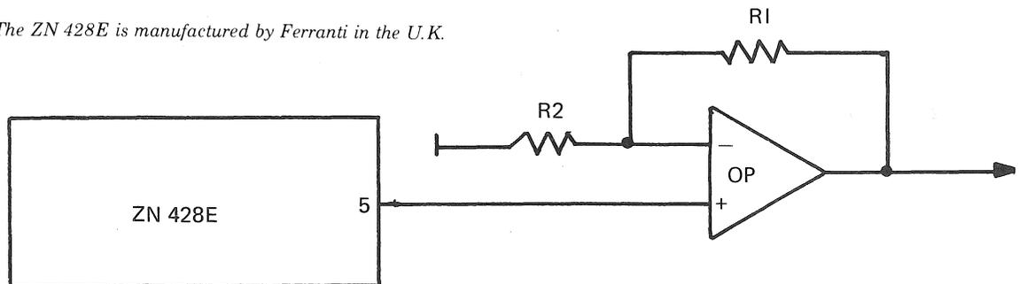
*Figure 3.2 D/A Block Diagram*
