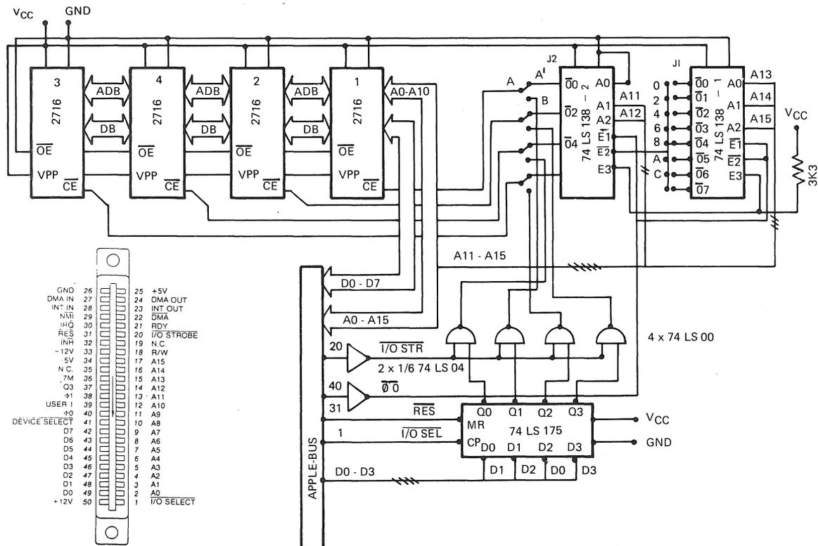
Figure 5.1 Schematic of the Eprom RAM Board
