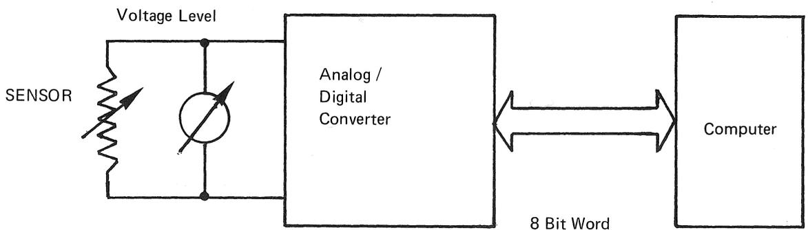
Figure 3.10 Block Diagram of the A/D Converter
