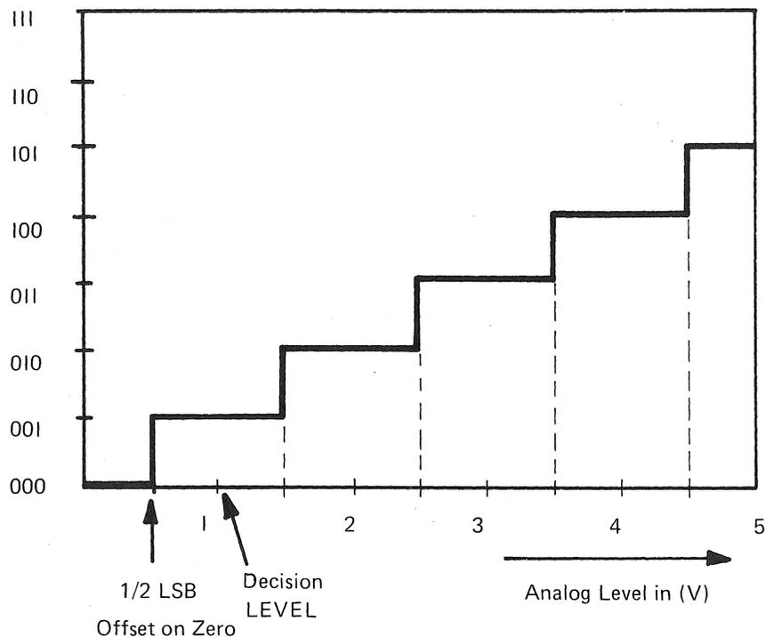
Figure 3.14 Quantized Input Signal
