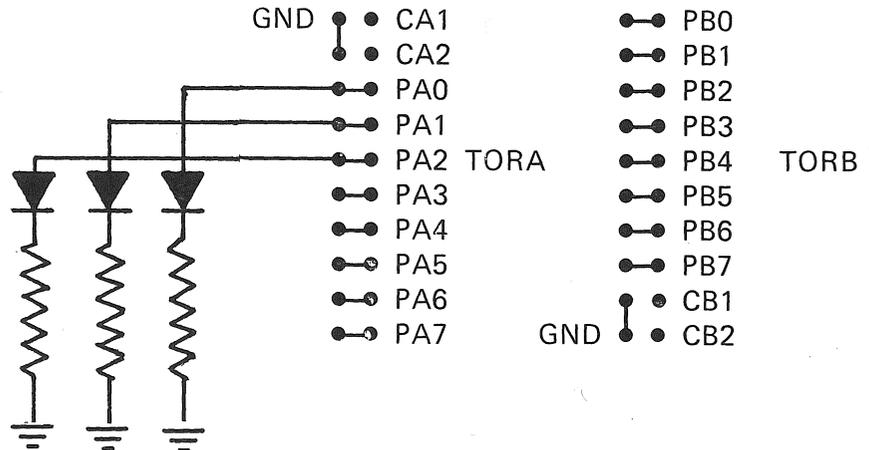
Figure 1.8 How to Connect LEDs to the Port
