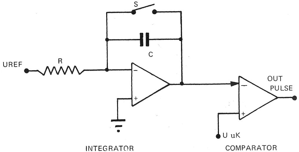
Figure 3.11 Schematic of the Integrator/Comparator
