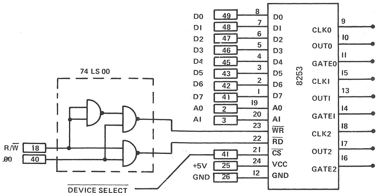
Figure 8.2 8253 Pin Connections
