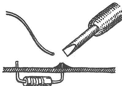
4. Remove the iron immediately and let the part cool. If a wire is being soldered, hold it still until the solder becomes cloudy and cool, or else an incomplete connection may result.
