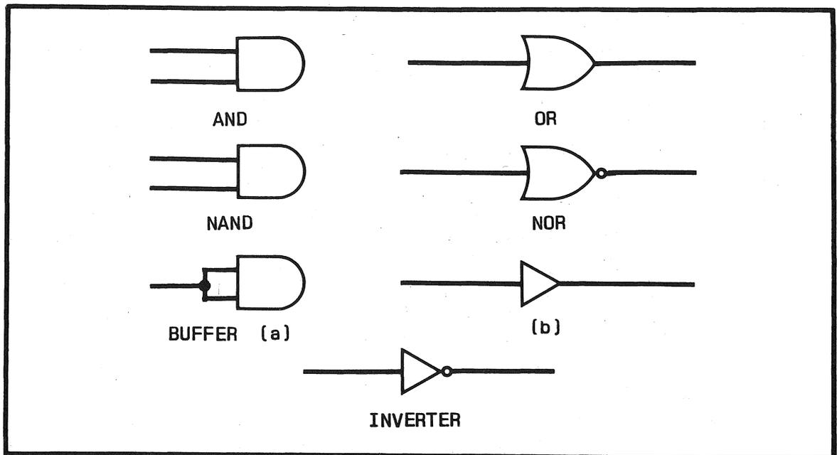
These symbols represent integrated circuits, those multiple lead, buglike packages that handle the bulk of the work in the computer. Briefly, these are logical building blocks. Sometimes there are several blocks in one integrated circuit, and these various blocks may be scattered throughout the circuit diagram. This can be confusing when actually building a circuit, but since pin (lead) numbers are given, you only have to remember where you put the part.
