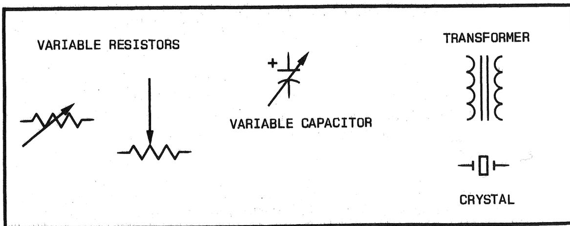
The first is a transformer, whose job it is to take current fed into one coil and induce that current, into a second coil. An iron or ferrite center (the parallel lines in the symbol) aids in efficient transfer of that current.
