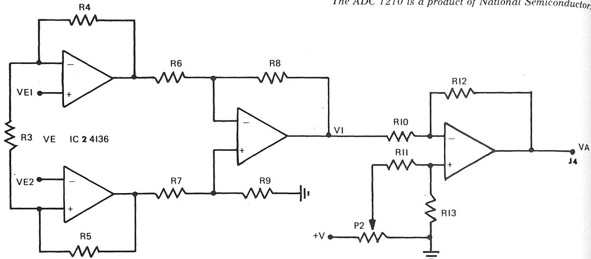
Figure 3.27 Instrumentation Amplifier Schematic
