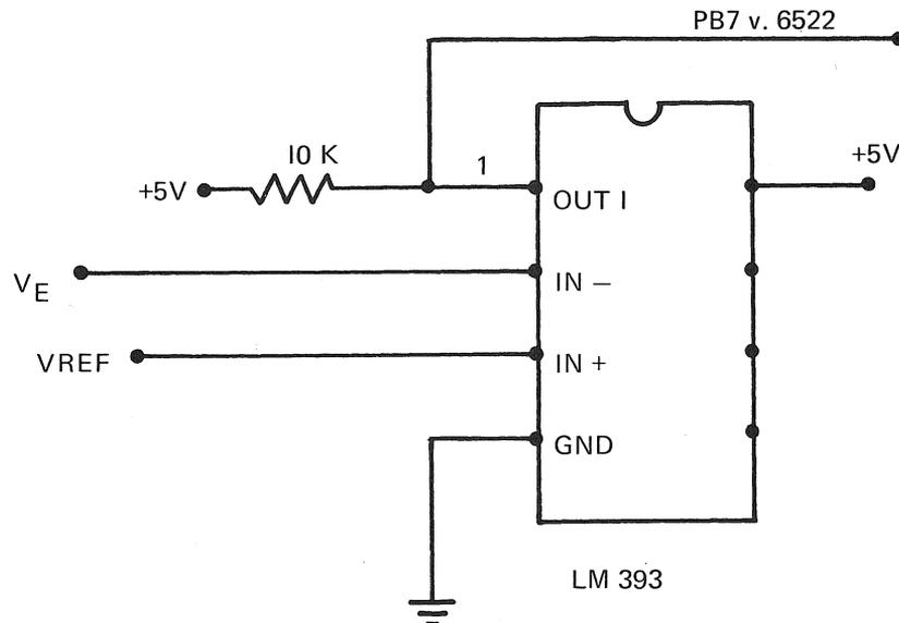
Figure 3.19 Block Diagram of the LM393
