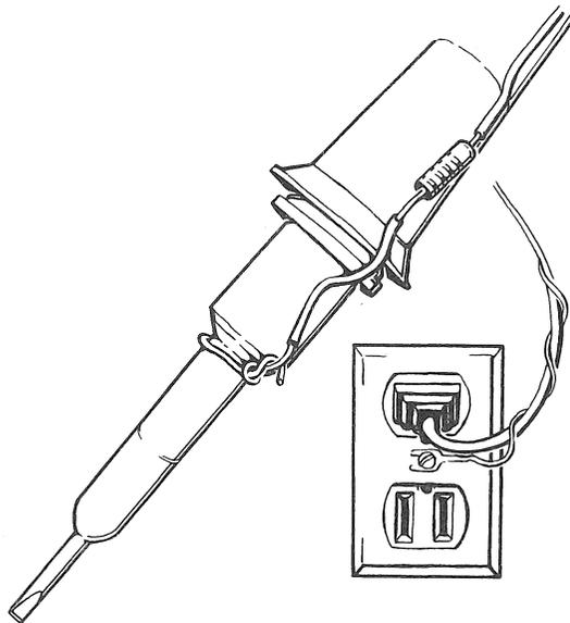
*Grounding a Soldering Iron*
