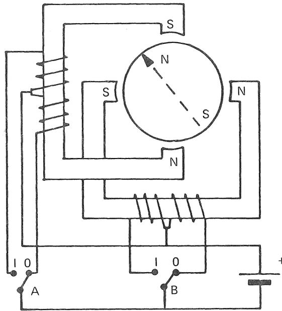
Figure 9.3 Step Motor Movement
