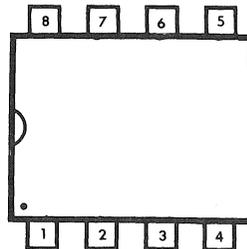
*Dip-type IC Pin Numbering (8 Pins)*
