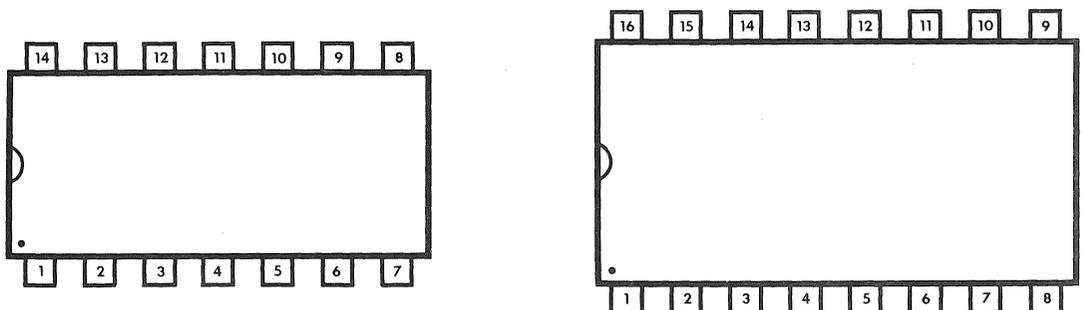
*14- and 16-Pin Dip IC Pin Numbering*
