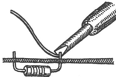
3. In the olden days, the rule was 'heat the parts, not the solder'. Forget it. Make sure the iron is no hotter than 40 watts (and remember never to use a soldering gun) and that the parts you are about to solder are very clean. Place the iron against the part, making as much contact with it as possible along the angled tip of the iron. Place the end of the solder at the junction of the iron and the part, and flow just enough solder to make a clean, shiny, flowing connection.
