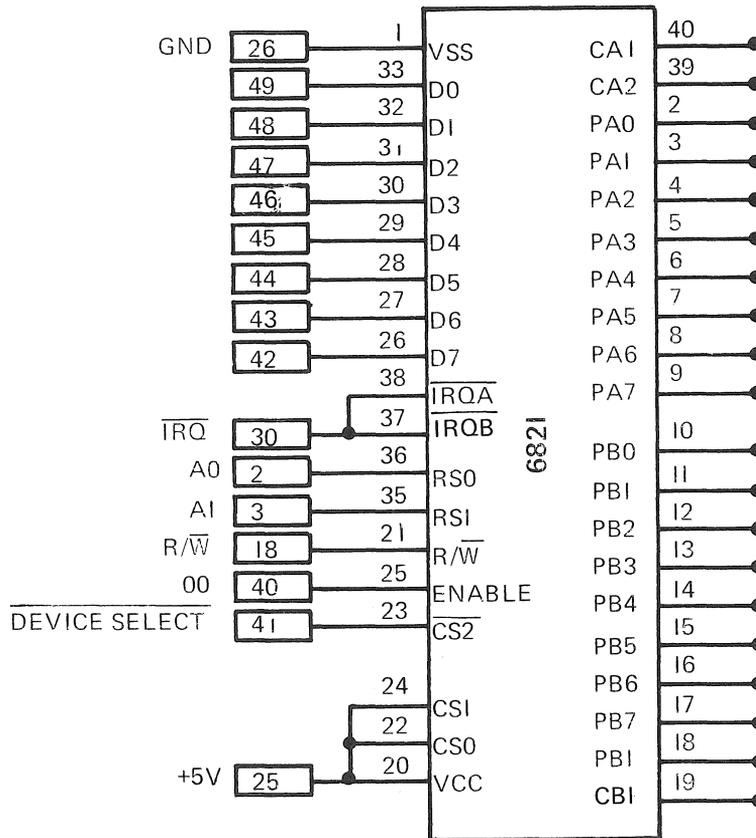
Figure 8.21 Pin Configuration of the 6821
