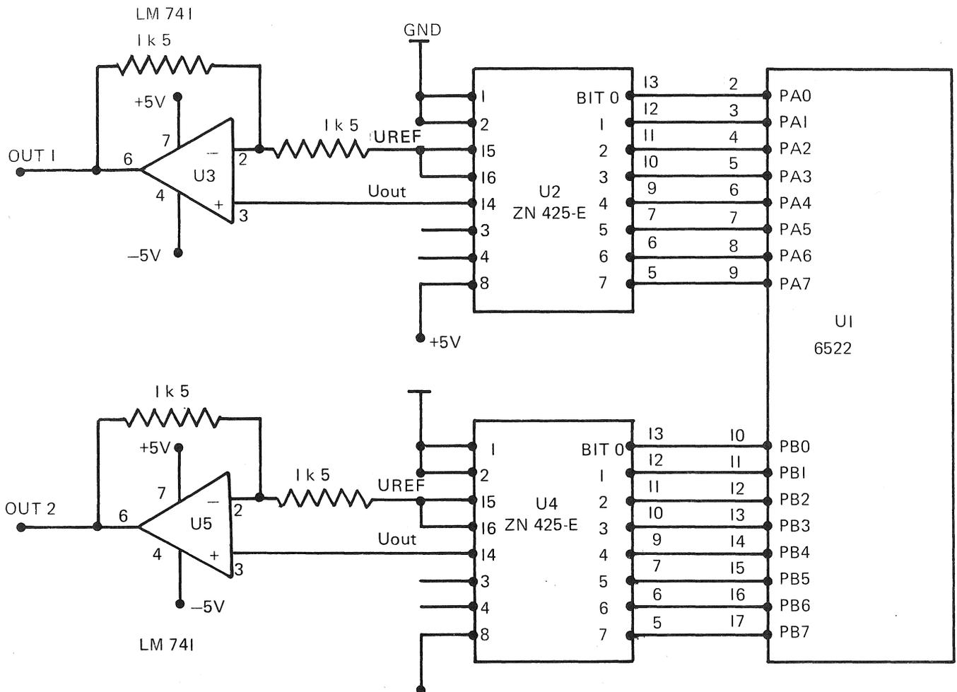
Figure 3.22 Connecting DAC ZN 425E's to the 6522
