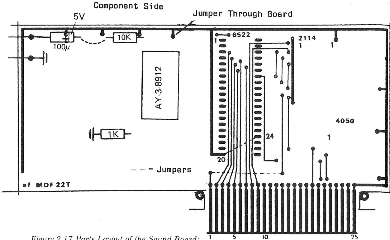
Figure 2.17 Parts Layout of the Sound Board
