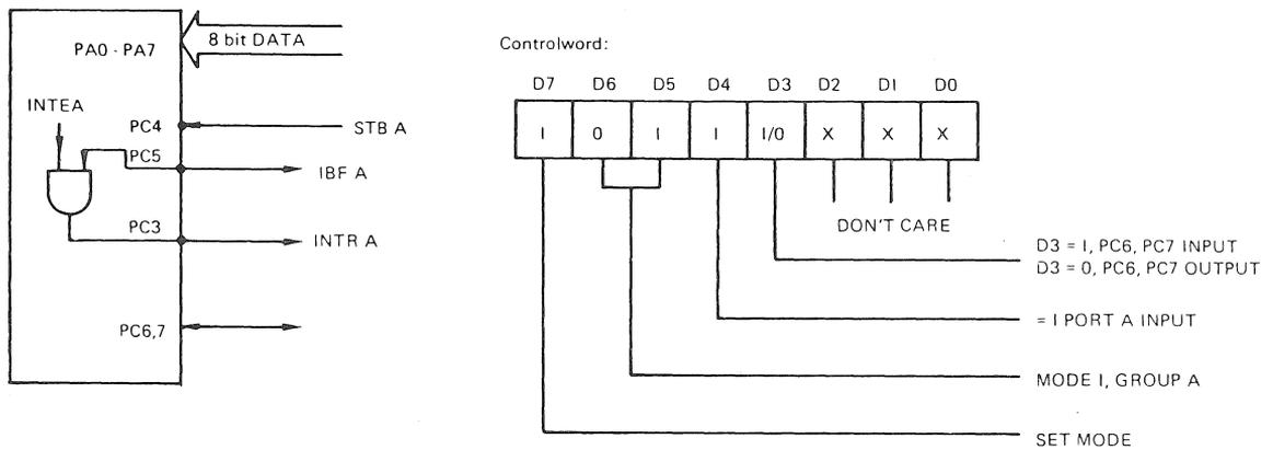
Figure 8.18 Output Signal Definition
