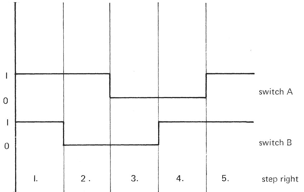
Figure 9.5 Right Turn Timing Diagram
