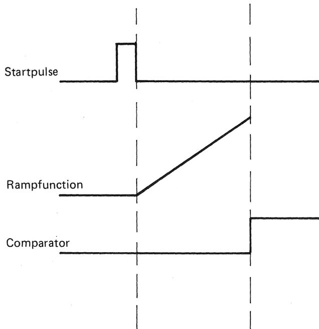
Figure 3.12 Digital Conversion with a RAMP Function
