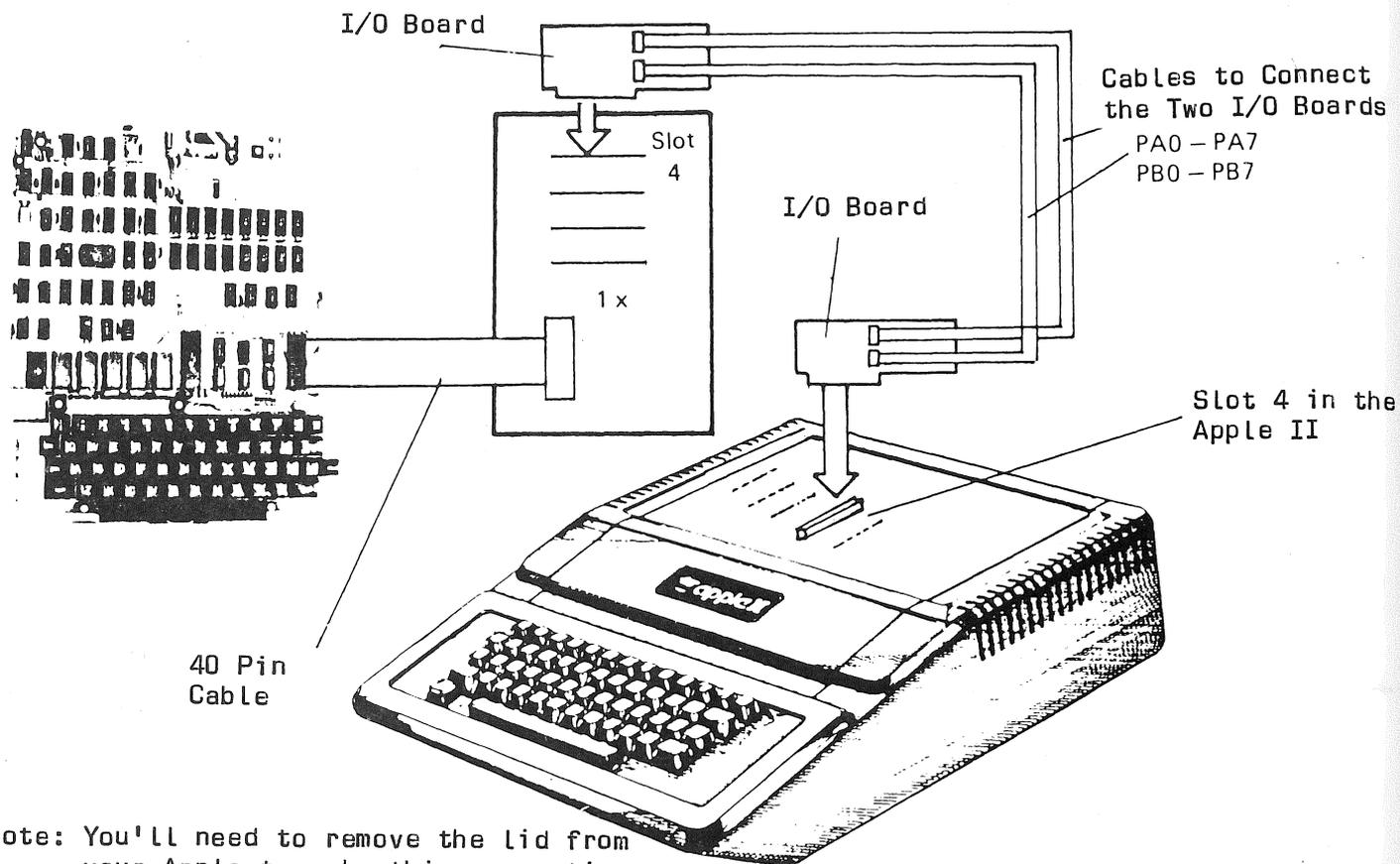
Figure 7.1 Block Diagram
