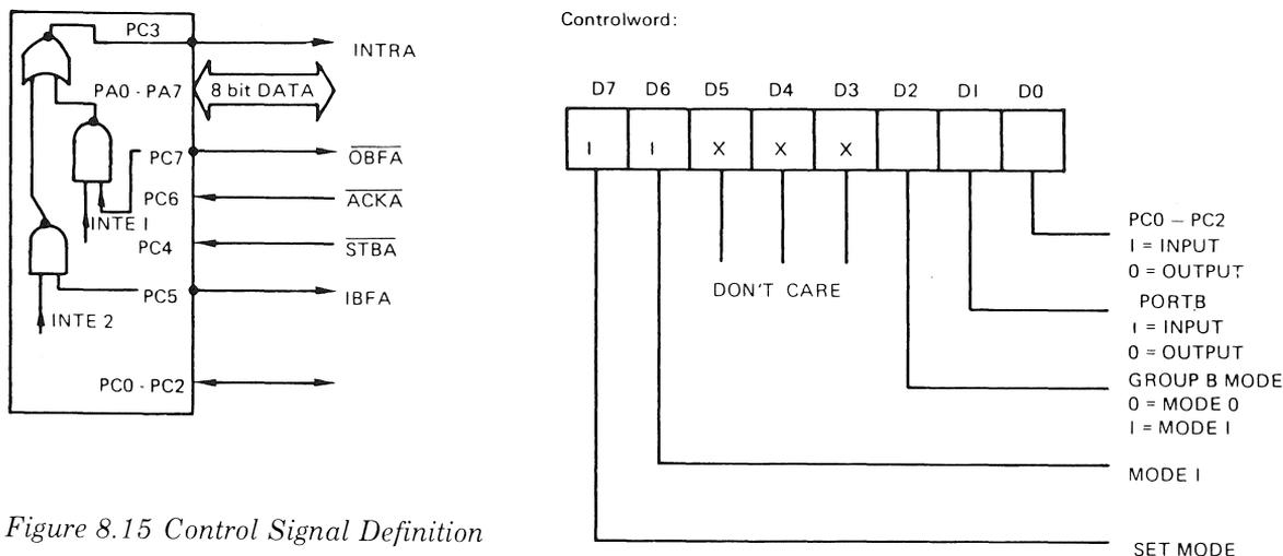
Figure 8.15 Control Signal Definition
