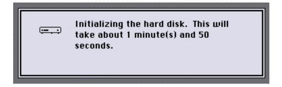
HD Install is now formatting the virtual Profile hard drive for MacWorks, by erasing all the sectors on it, and installing the MFS file system.
