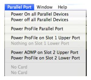
This menu allows you to switch power on individual ProFile hard drives, and ADMP printers, or all parallel port attached devices simultaneously.
